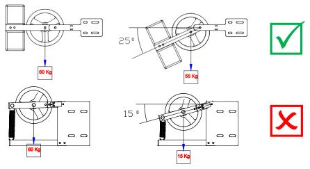
Even if the rope stretches in a weighted tensioning system, the weight changes are around 10%.
